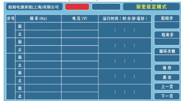
The gradient Settings page can set the required voltage and frequency Run time, initial step, end step
