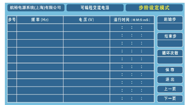
Step setting page can set the required frequency, voltage, Run time, initial step, end step, and number of cycles
